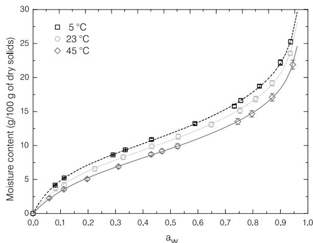
Figure 1. Adsorption isotherms of rice flour for a temperature range of 5 to 45°C. Open squares: 5°C, open circles: 23°C, open diamonds: 45°C. Modified GAB fits are shown on the graph (dashed line: 5°C, dotted line: 23°C, solid line: 45°C).
