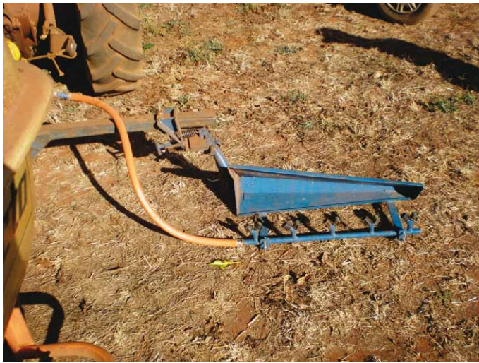
Figure 1. Device for pesticide application (wing) on the lower inner part of the canopy of coffee crops.
