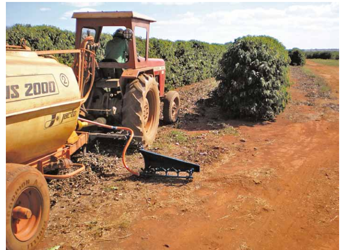
Figure 3. Details of the developed device coupled to the sprayer in the field.
