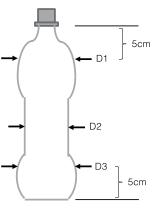
Figure 1. Schematic of the PET probe indicating diameters D1, D2 and D3.
